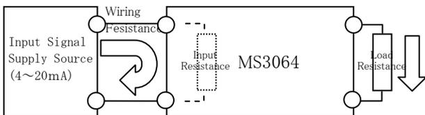
\*Input resistance for voltage output type is fixed to approx. 250 Ω (for 20mA DC input).
