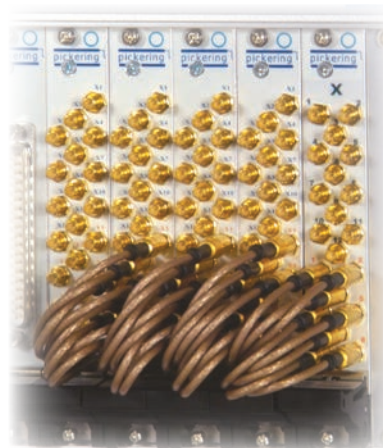
Optional Y-axis loop-thru allows easy expansion. Shown here is a 60x8 RF matrix with over 200 MHz bandwidth.
